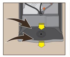
5 Clean the trash bin and drip pan: With the machine door open, remove the trash bin and drip pan forwards. Empty the coffee grounds and water.
