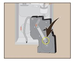
6 Push down the bolts for the crank drive on the back of the brewer.
