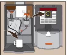
2 Place the rinsing cup under the spout. Then press the program button in the door.
