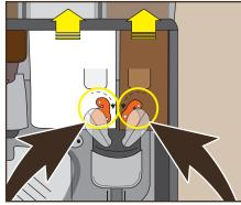
8 Seal both caps and remove the product container upwards.
