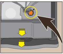
2 Remove the trash bin and drip pan and unscrew the orange screw cap.
