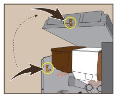
Open the machine door. Remove the service key from the holder on the left wall of the housing and start up the machine.
