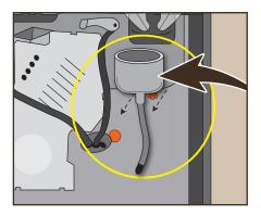
**10** Fully release the tube at the delivery outlet. Remove the complete mixer and tube forwards.
