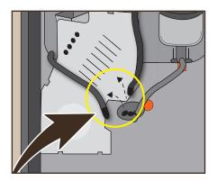
4 Remove the delivery tube on the left and the coffee tube directly next to it, and allow them to hang down loosely.
