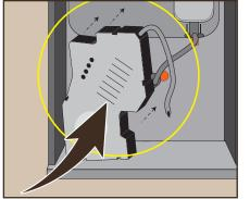
Clean the coffee strainers under running water and thoroughly dry the brewer. Install the brewer in reverse order between the red retaining lugs.
