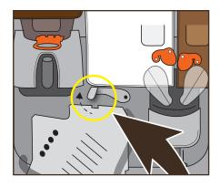
Push the brewer's retaining brackets upwards.
