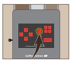
Press button 4 to select the rinsing program. Press button 10 to confirm that the drip pan is empty. Press button 10 to confirm that the water is OK.
